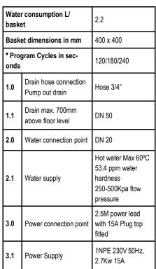
\*For connection to cold water and/or short basket exchange times, the wash cycles may increase to achieve hygienic final rinse temperatures.
